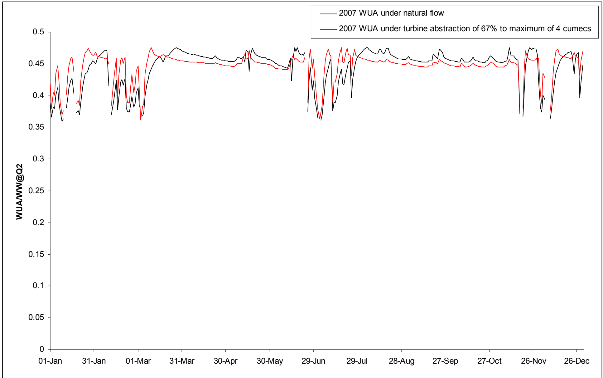
(xxiv) Impact of a turbine take of 67% of river flow above Q90 in 2007, up to a maximum of 4 cumecs, on the WUA/WW@Q2 for 0-7cm trout
