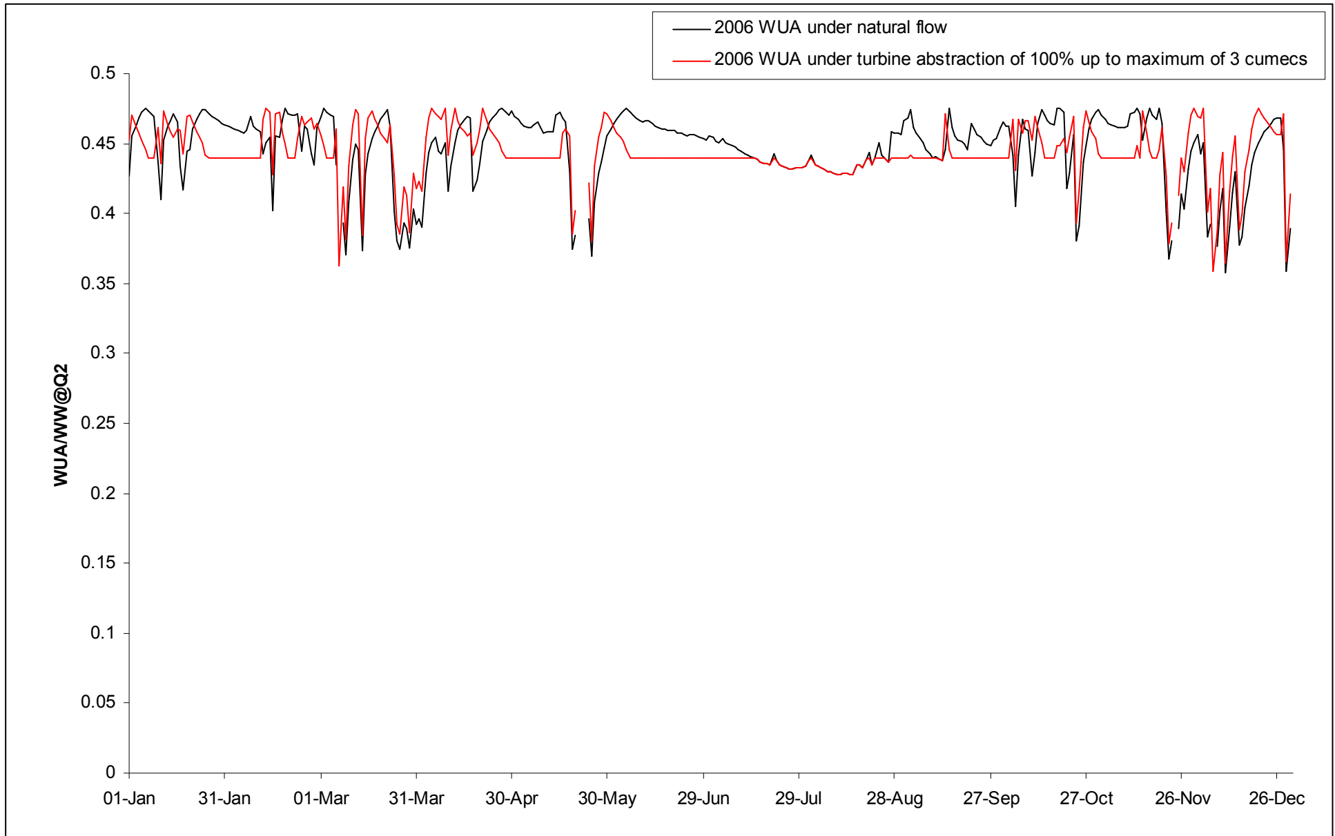
(iii) Impact of a turbine take of 100% of river flow above Q90 in 2006, up to a maximum of 3 cumecs, on the WUA/WW@Q2 for 0-7cm trout.
