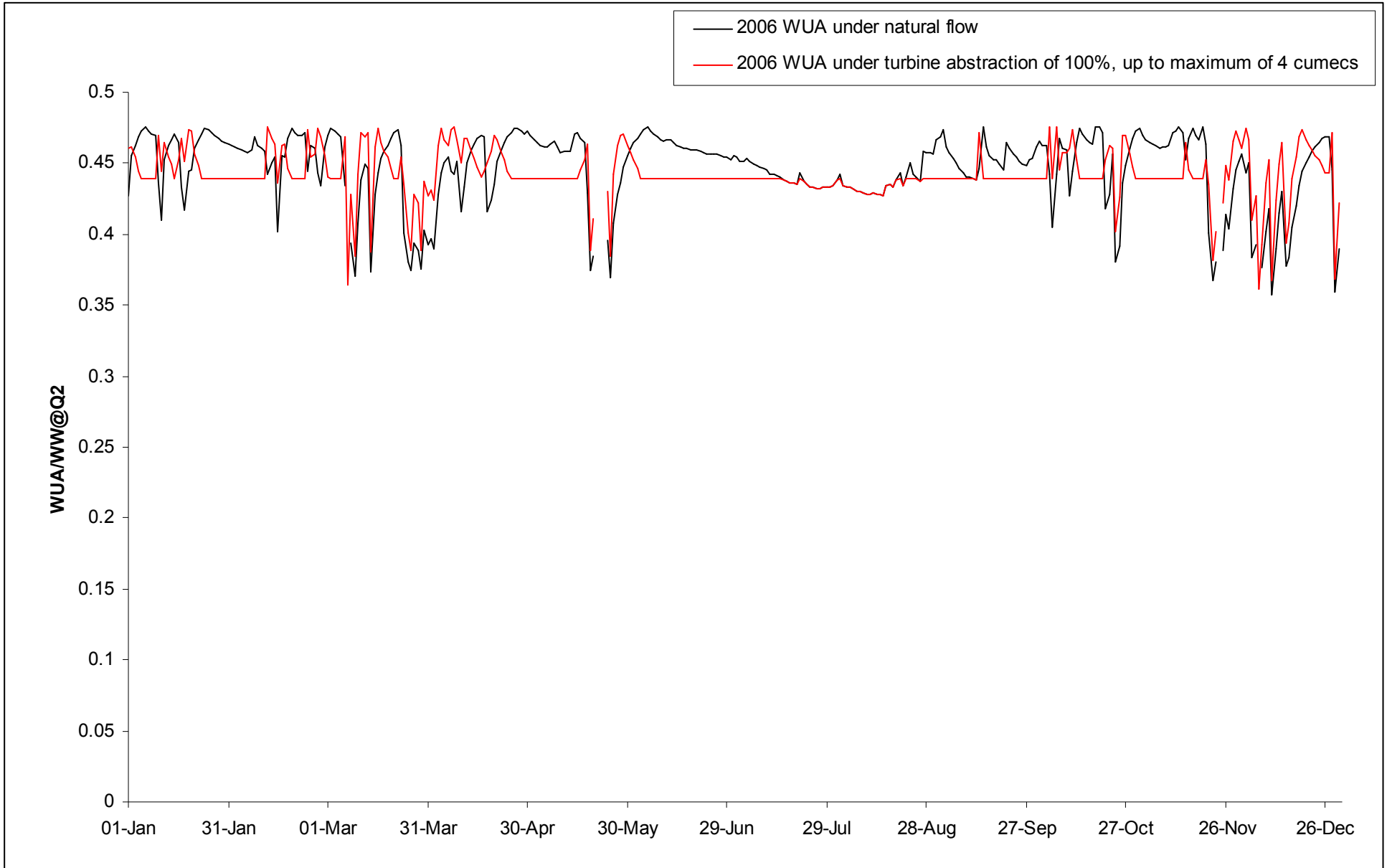
(vii) Impact of a turbine take of 100% of river flow above Q90 in 2006, up to a maximum of 4 cumecs, on the WUA/WW@Q2 for 0-7cm trout.
