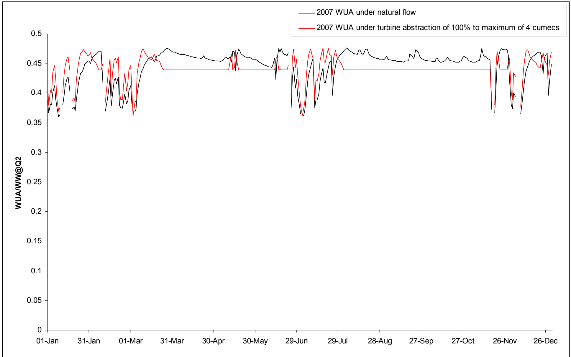
(xxiii) Impact of a turbine take of 100% of river flow above Q90 in 2007, up to a maximum of 4 cumecs, on the WUA/WW@Q2 for 0-7cm trout
