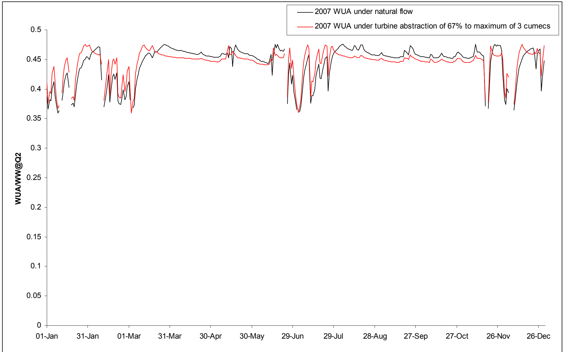
(xxii) Impact of a turbine take of 67% of river flow above Q90 in 2007, up to a maximum of 3 cumecs, on the WUA/WW@Q2 for 0-7cm trout
