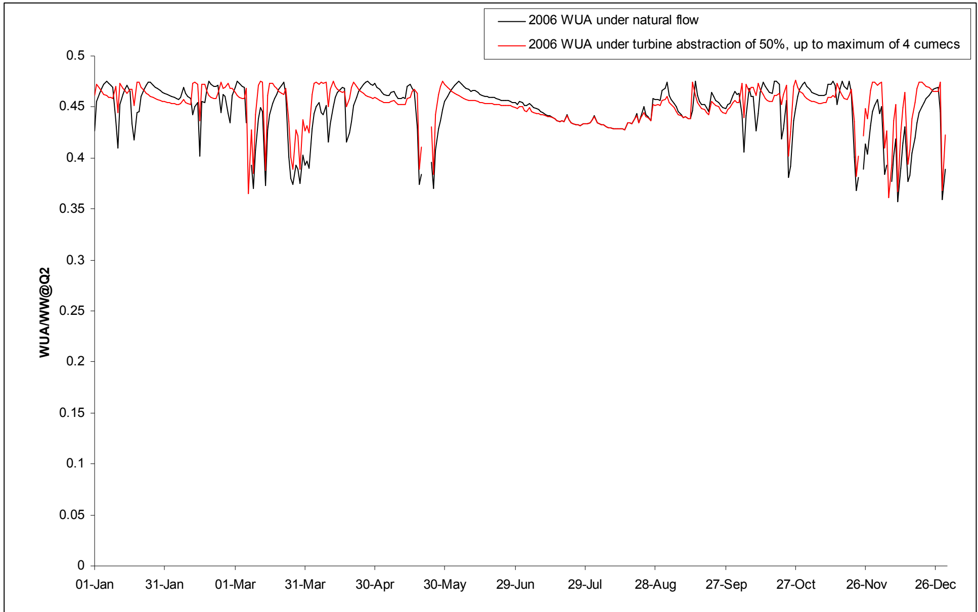
(x) Impact of a turbine take of 50% of river flow above Q90 in 2006, up to a maximum of 4 cumecs, on the WUA/WW@Q2 for 0-7cm trout.
