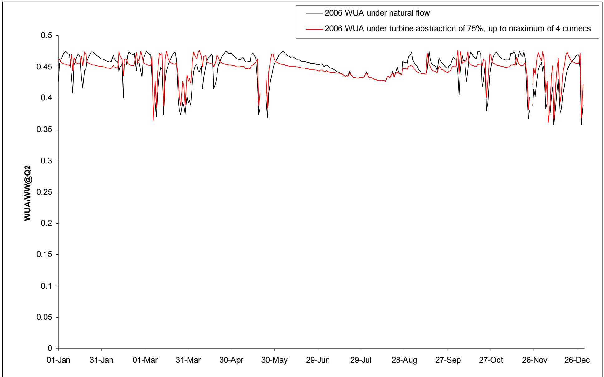
(viii) Impact of a turbine take of 75% of river flow above Q90 in 2006, up to a maximum of 4 cumecs, on the WUA/WW@Q2 for 0-7cm trout.
